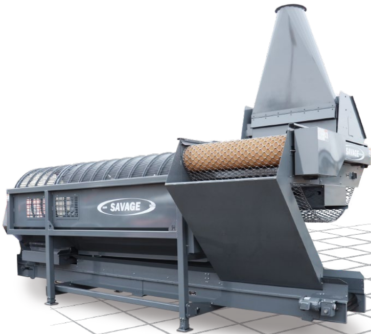
60-inch Stick Remover with Pre-Vac Mounted on Cleaning Reel with Trash Conveyor
