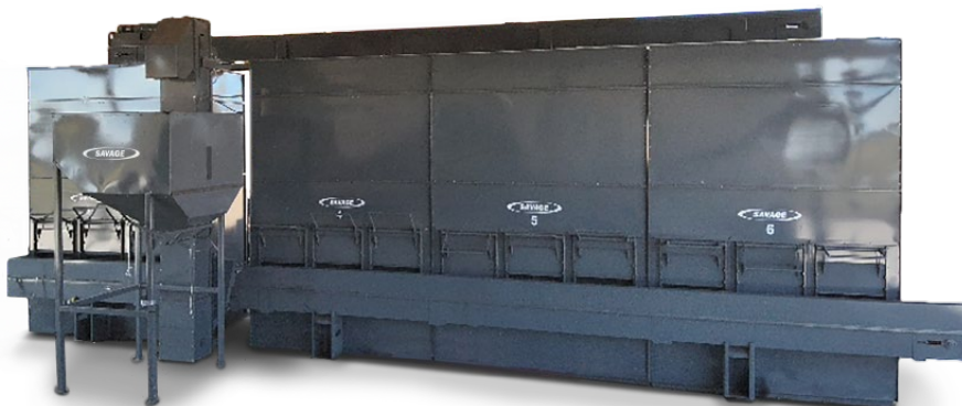
Drying Bins with Bucket Elevator and Hopper
